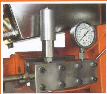
Stainless steel pump-head. Integrated cooling for plunger-seals.
