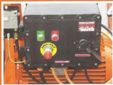
Cast electrical Eex box with main switch, star delta starter and overload relay.
