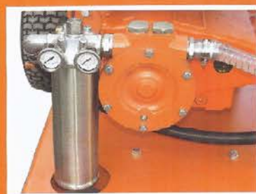
Integrated booster pump & filter system.
